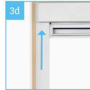
3d Continue to push the siderail until it is fully inserted behind the cassette.
